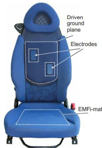
Figure 5. The co-driver seat featuring capacitive electrodes at the backrest and an additional acceleration sensor (EMFi-mat) in the seat [87].
