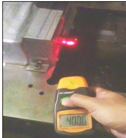
Figure 13. Rotation of spindle is measured by laser type Tachometer.
