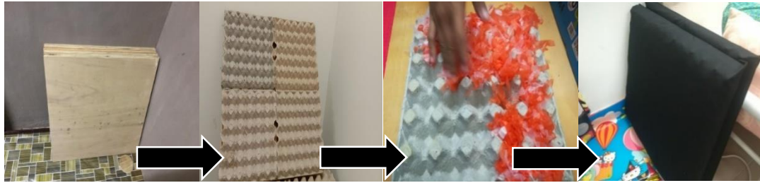
Figure 5. Absorption panels (egg trays with recycled plastics) design stages.
