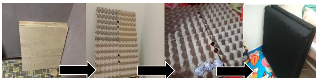
Figure 4. Absorption panels (egg trays with recycled papers) design stages.
