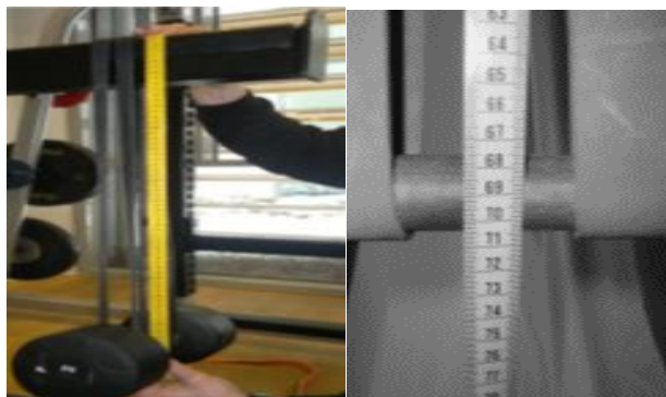
Figure 3: Calibration of elastic bands using protocol by Shoepe et al. (2010)
