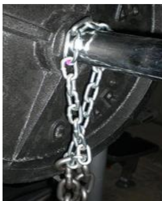
Figure 4: The support chain goes thru any link in the training chain and connects to form a complete loop that slips over the ends of the bar
