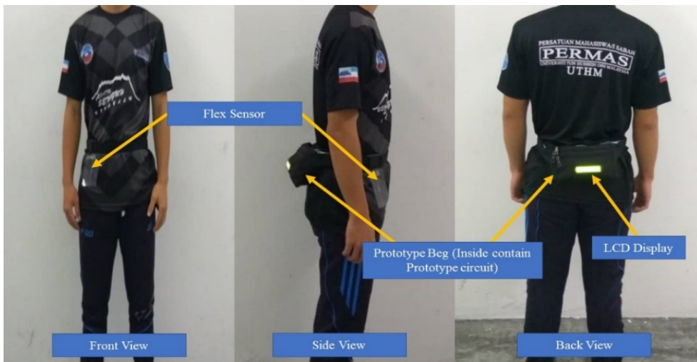
Figure 12: Placement of the proposed device within the porch and the flex sensor on the subject's hip
