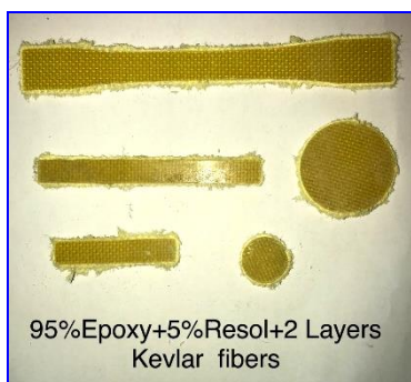
Figure 6. Tensile, toughness, and hardness test samples with different types of fibers (carbon, glass, Kevlar).
