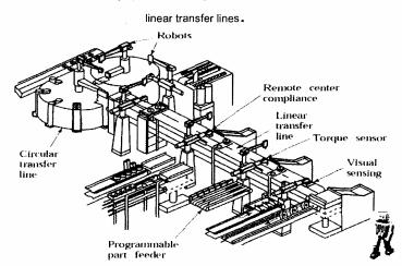
Automated assembly operations using industrial robots and circular and
