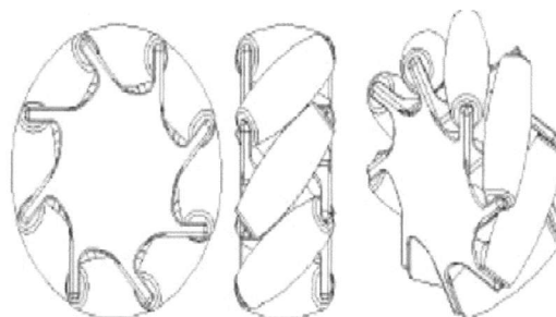
Fig 1: Mecanum wheel based on Ilon's concept. Source from [1].
