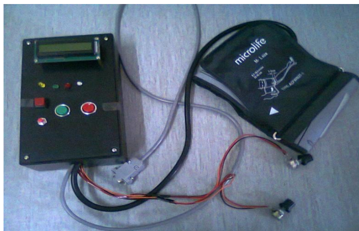
Figure 7. Our developed hypertension diagnosis kit.
