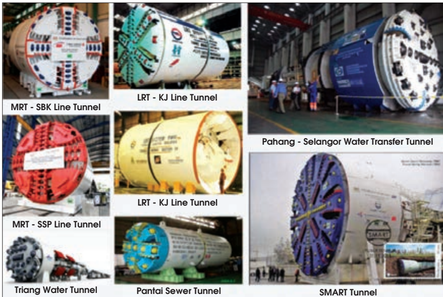
Figure 6: TBMs employed in past tunnelling projects
