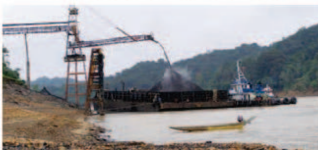
In Kapit, a barge is filled with coal via a conveyor belt
