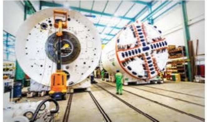
MRT Line 1 Tunnel Boring Machine under construction
