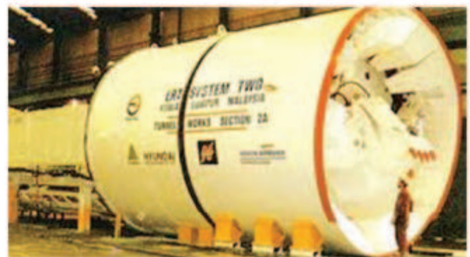
Open Shield for Putra Line 1996: Picture courtesy of Tuan Haji Sabre
