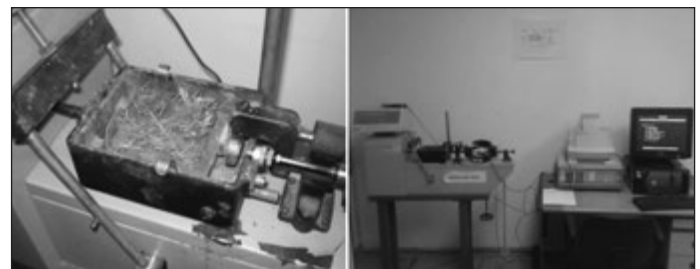
Figure 6: Soil Block Placed in the Shear Box
