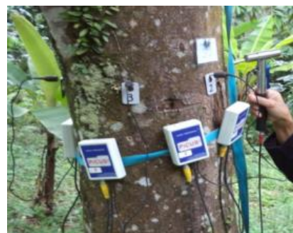
Figure 2 The set-up of acoustic tomography in agarwood imaging [3]
