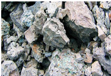
Figure 3.2: Chunky raw palm slag from local palm oil industry
