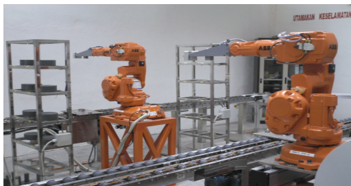
Fig.2. Storage buffers and robots used on automated production line.
