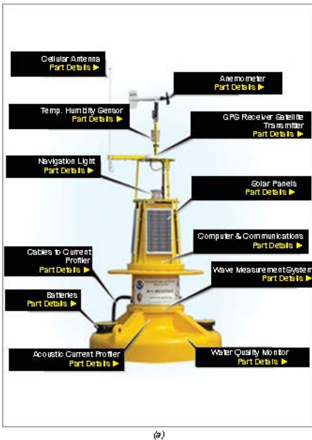
Figure 2: Sensor placements on (a) CBIBS Buoy and (b) Oceanographic buoy by Sirio d.o.o. Koper
