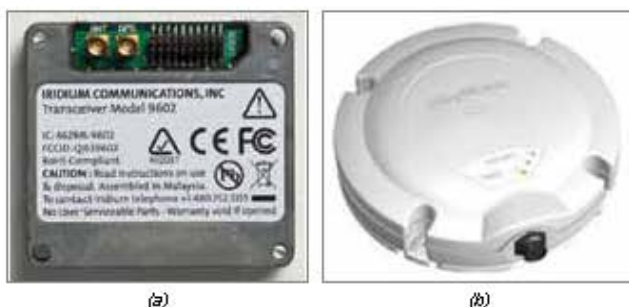
Figure 3: Satellite transceiver for (a) Iridium satellite and (b) Inmarsat D+ satellite
