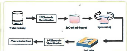
Figure 2: Zinc Oxide Thin Film Pressure Sensor Preparation
