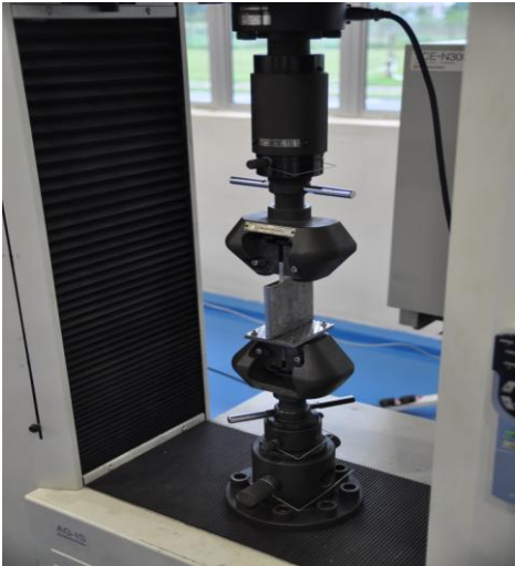
Figure 3. Specimen mounted on UTM machine.
