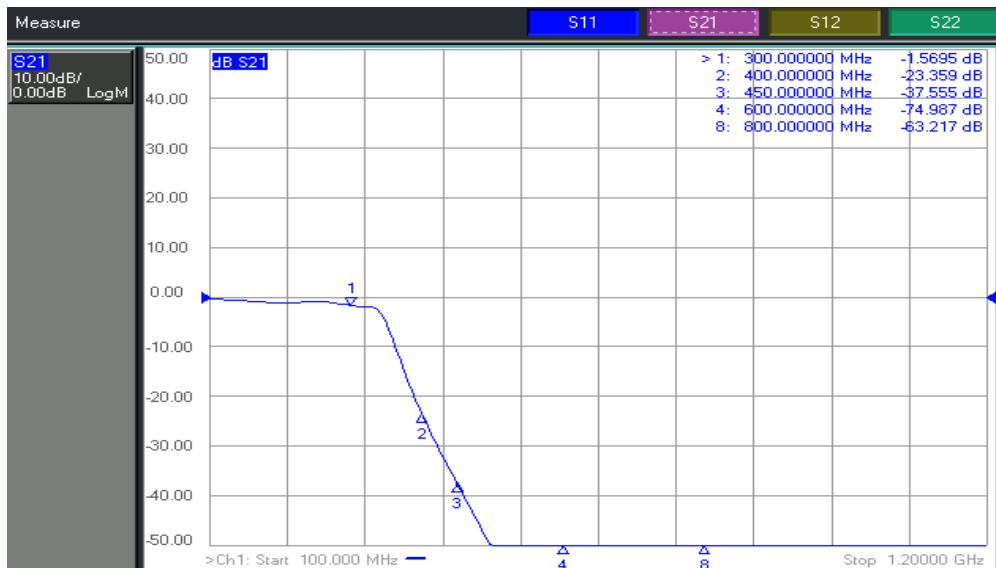
Fig 8. Simulation S21 results for Butterworth low pass filter
