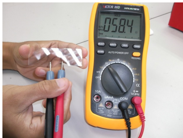
Figure 3. Indium tin oxide coated glass slide, 30 ~ 60 \Omega /sq surface sensitivity
