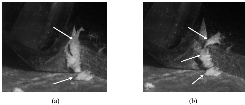
Figure 6 Video footages during chip formation of side end milling GFRP composites at N = 300 RPM, f_r = 0.32 mm/rev and A = 0^\circ
