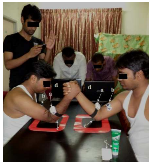
Figure 1. Experimental setup for EMG data recording: a) wireless EMG sensor attached within the daughter board; b) active electrodes; c) reference electrodes; d) Bluetooth-enabled laptop computers for recording the EMG signal within a 2 meter range; e) skin cleaning gel and alcohol swabs.
