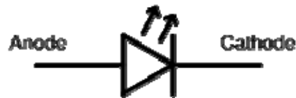
Figure 1.3: LED Schematic Symbol
