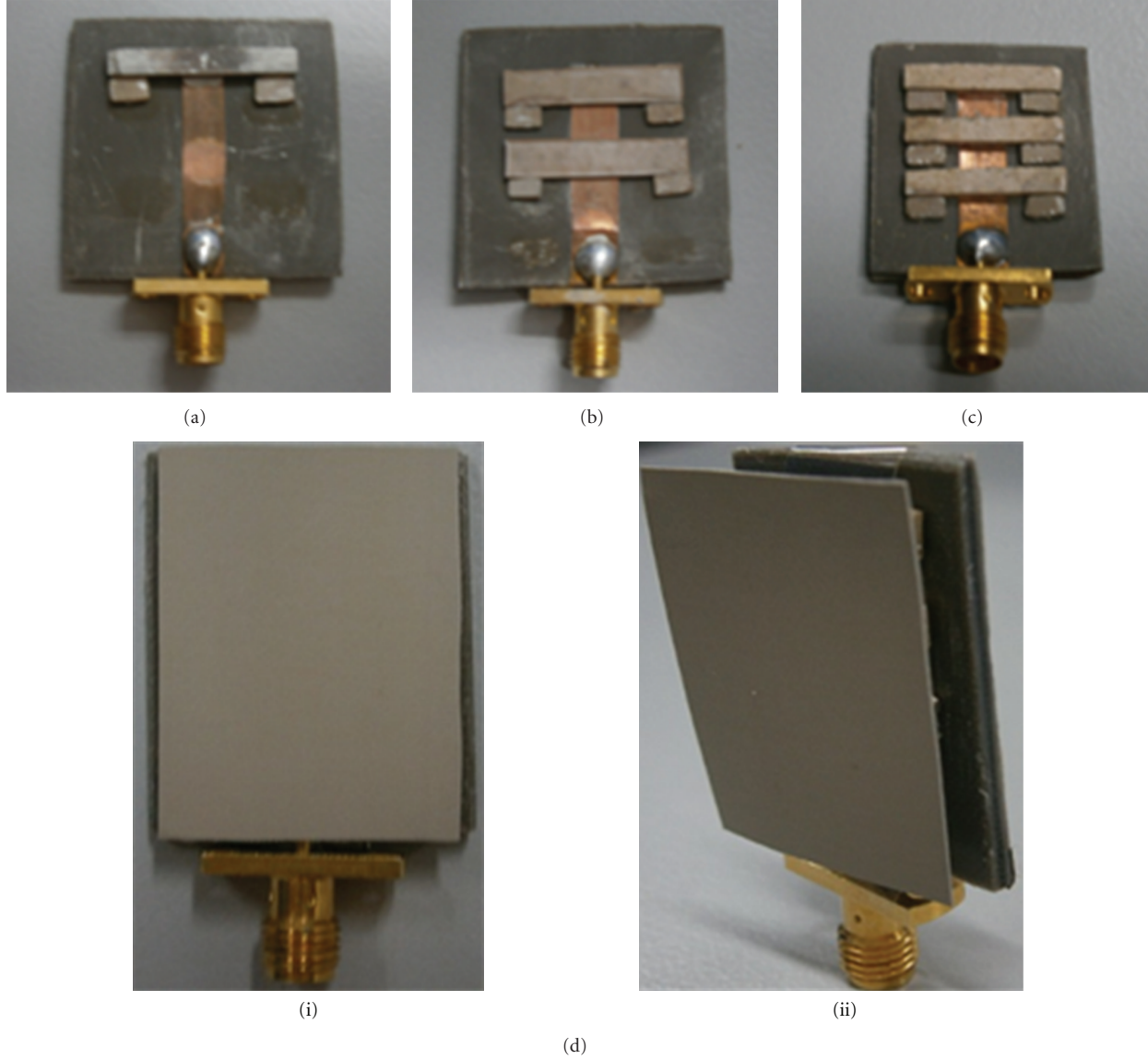
FIGURE 6: Photograph of fabricated BiT array antennas (a) two BiT ceramic elements (b) four BiT ceramic elements (c) six BiT ceramic elements (d) dielectric layer (i) front view (ii) perspective view.
