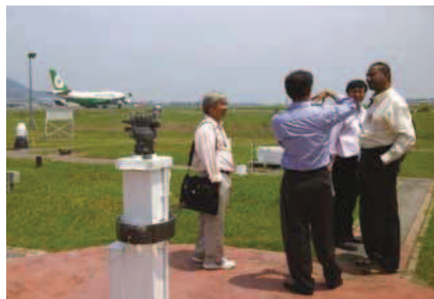
A theodolite equipment (in front) was on standby to record positions of a released balloon filled with helium, which was released to measure wind speed. In the background, a plane can be seen landing on the runway of Bayan Lepas Airport
