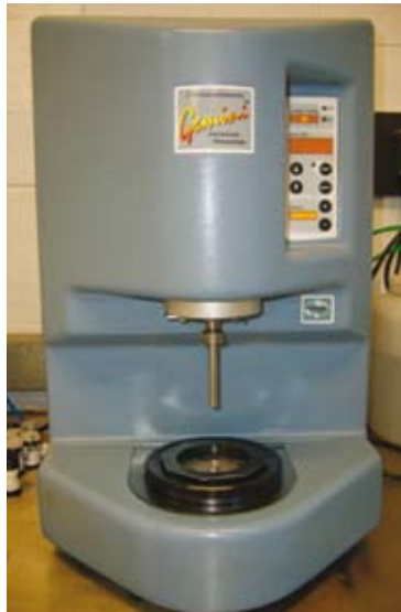
Figure 2: Dynamic shear rheometer (DSR)
