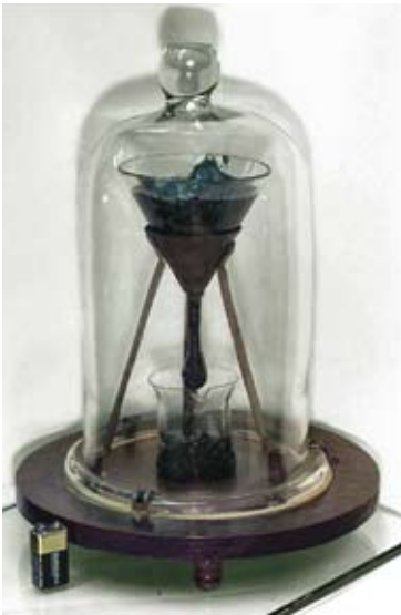
Figure 1: Pitch drop experiment [5]
