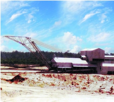
Figure 12: The classic dredge, an efficient mining machine in flat alluvial ground
