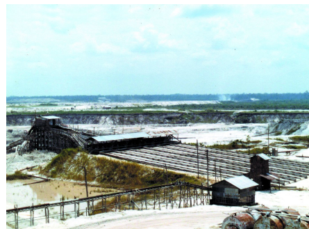
Figure 10: Palong, a giant sluice to collect tin ore
