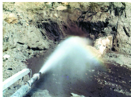
Figure 9: High pressure water jet or monitor breaking up the ore bearing earth
