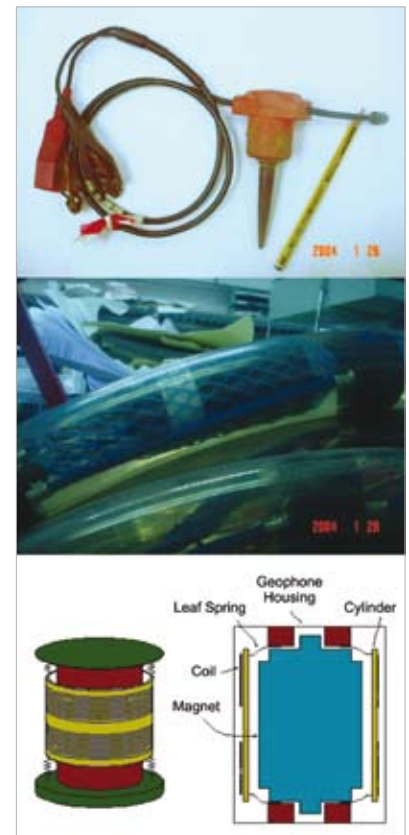
Figure 2: Geophone and its schematic details
