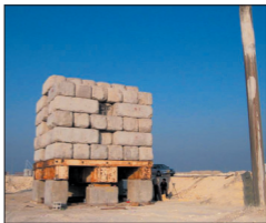
A static load test
