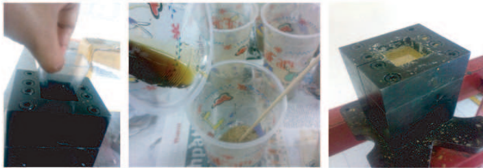
Figure 5. Fabrication process of the pyramidal microwave absorber.
