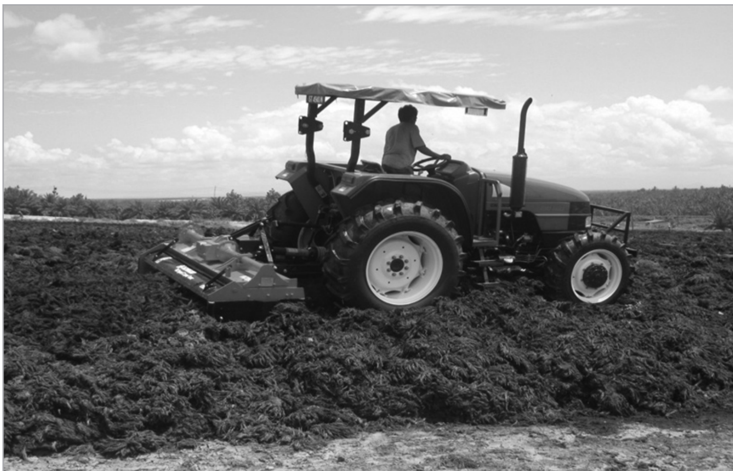
Figure 3: Empty fruit bunch-POME compost turning using tractor with macerator (Courtesy of Prestige Central Management Sdn. Bhd.)
