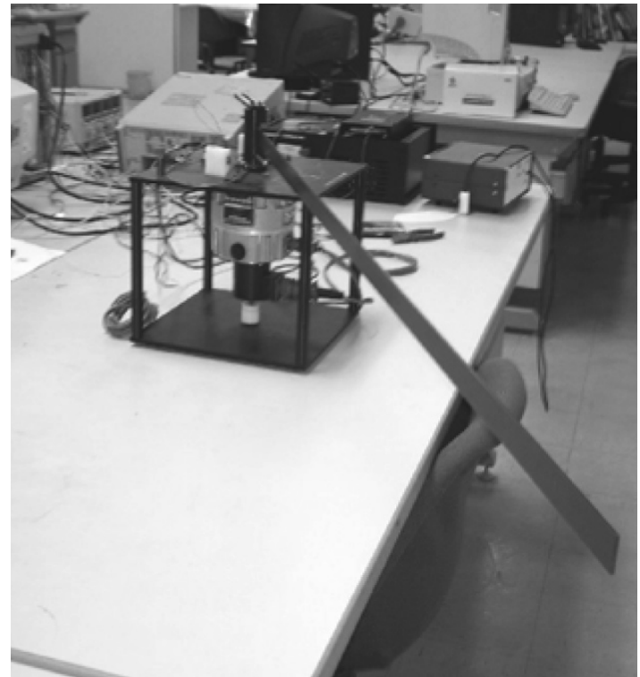
Figure 2: Actual flexible-link test bed in UTM
