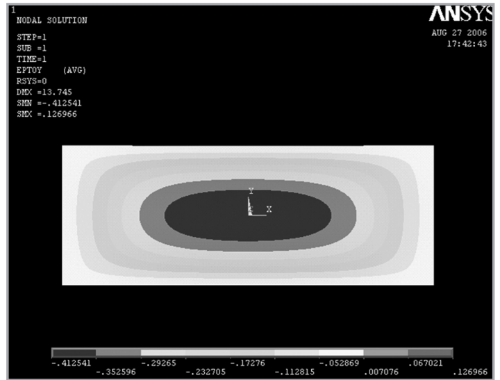
Figure 9: Gauge pattern on maximum strained area of substrate
