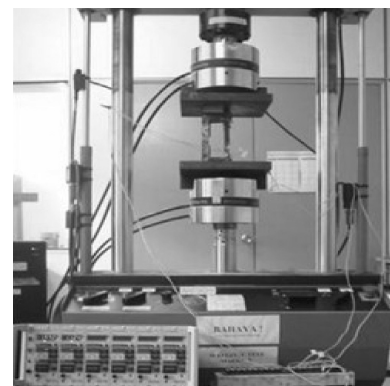
Figure 13: (a) Load Cell-B calibration fixture
