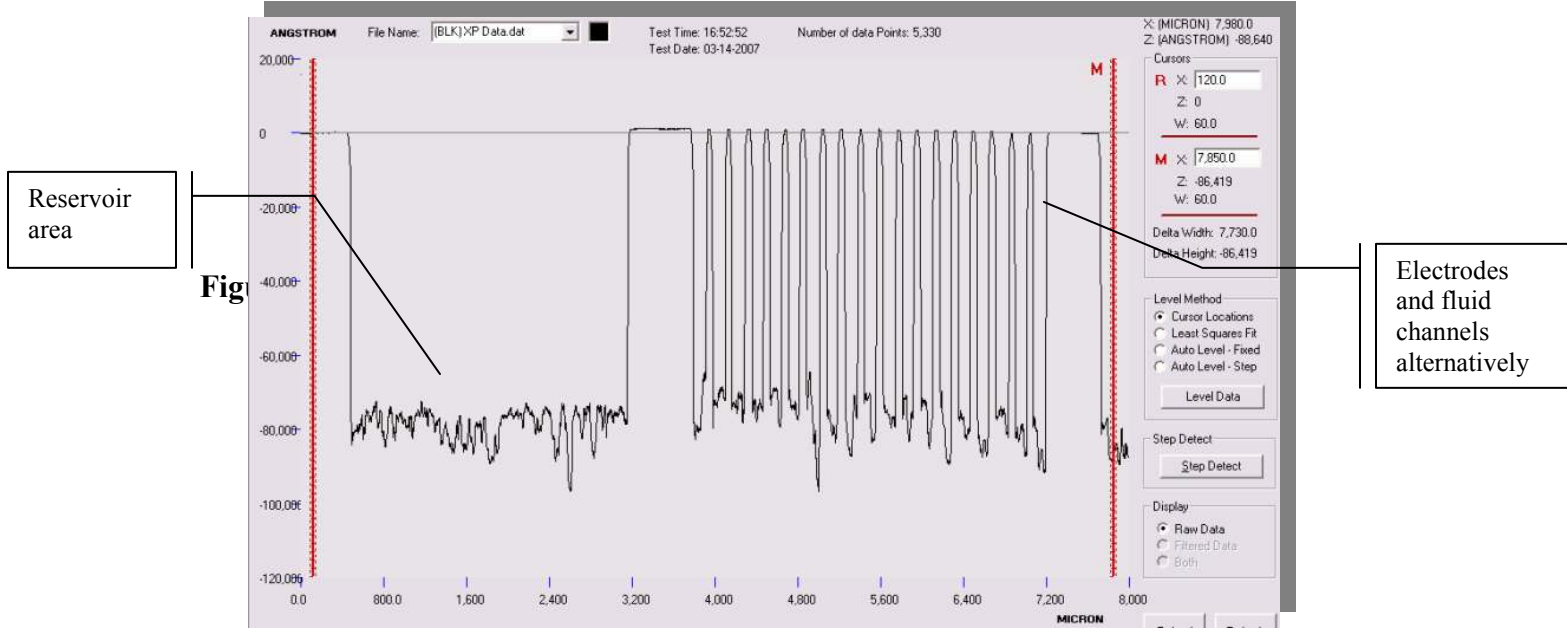
Figure 4.8: Surface profile of wafer B after 20 minutes in KOH 25% at 60°C
