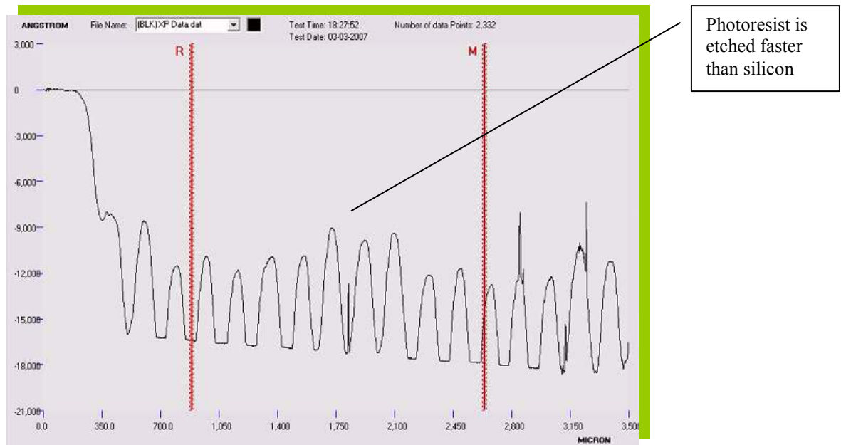
Figure 4.7: Surface profile after 5 minutes immersion in KOH for silicon etch with photo resist as mask
