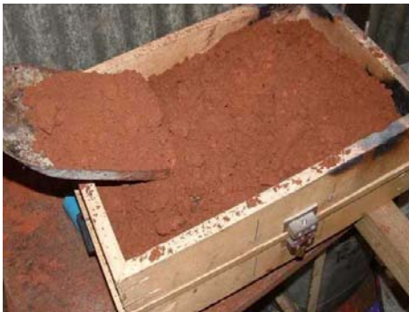
(c) Sand filling process
