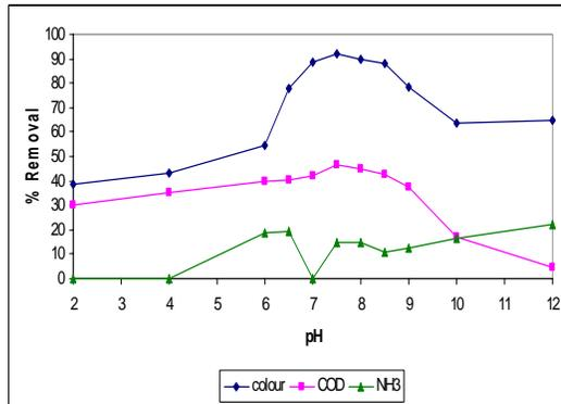
Figure 3: Percentage reduction of COD, colour and NH<sub>4</sub>-N vs pH. Tests performed with OpCD of PAC.
