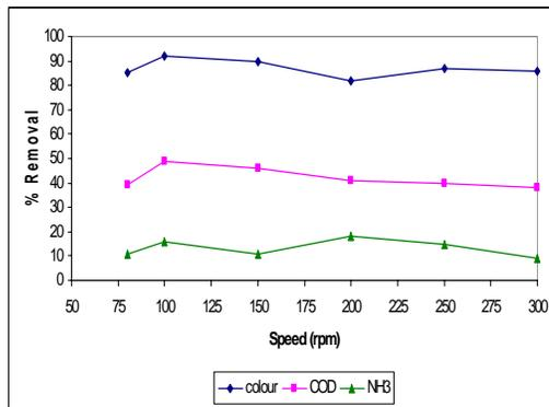
Figure 5: Percentage reduction of colour, COD and NH<sub>3</sub> vs speed of rapid mixing. Tests performed with OpCD and pH of PAC.
