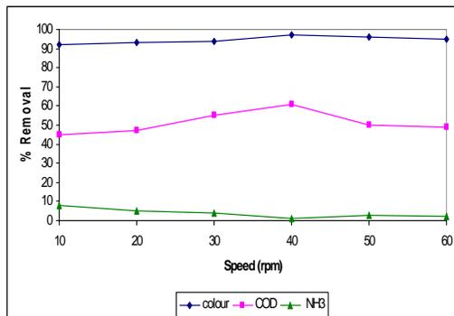
Figure 7: Percentage reduction of colour, COD and NH<sub>3</sub> in different speed of slow mixing. Tests performed with OpCD, pH and rapid mixing parameter using PAC.
