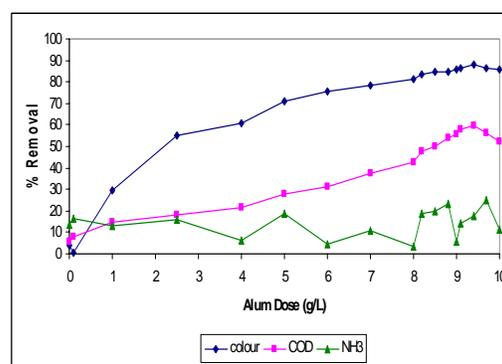
Figure 2: Percentage reduction of COD, colour and NH<sub>4</sub>-N vs alum dose. Test performed at neutral pH.
