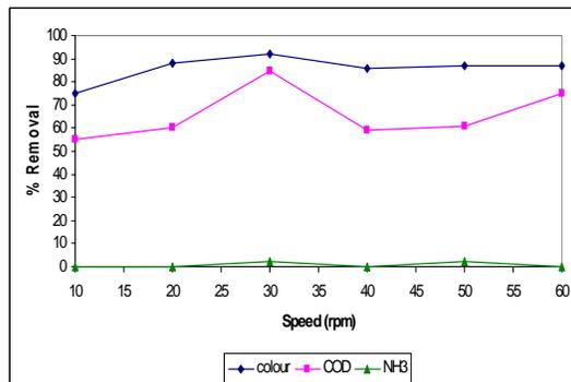
Figure 8: Percentage reduction of colour, COD and NH<sub>3</sub> in different speed of slow mixing. Tests performed with OpCD, pH and rapid mixing parameter using alum.
