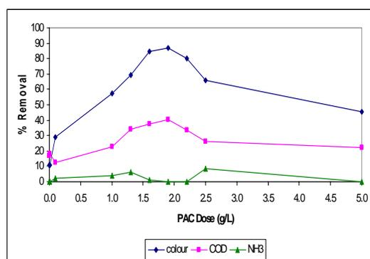
Figure 1: Percentage reduction of COD, colour and NH<sub>4</sub>-N vs PAC dose. Test performed at neutral pH.
