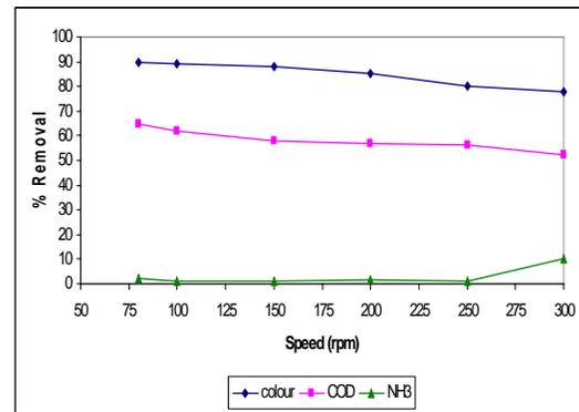
Figure 6: Percentage reduction of colour, COD and ammonia vs speed of rapid mixing. Tests performed with OpCD and pH of alum.
