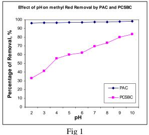
For the sulphuric acid treated bagasse (PCSBC), the dyes adsorption was significantly change over the pH value of 4 to 7. The lowest percentage of dye removal was recorded at pH 2 (52.2%). At the pH range 7 to 10, the percentage of removal was almost remains constant.
