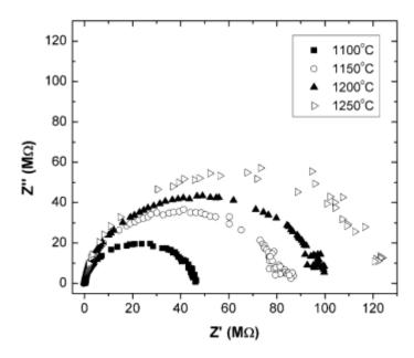
Figure 8. Nyquist plots under 300°C for calcium monosilicate sintered at different temperatures.
