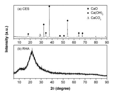
Figure 3. XRD result of calcined rice husk and calcined eggshell.
