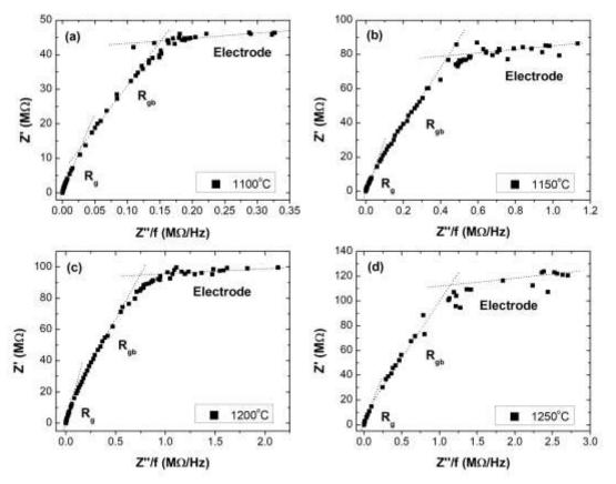
**Figure 9.** Alternate representations of impedance spectra under 300°C for calcium monosilicate sintered at different temperatures.
