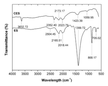
Figure 2. FTIR result of raw eggshell and calcined eggshell.
