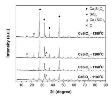
Figure 4. XRD result of sintered samples at different sintering temperatures.
