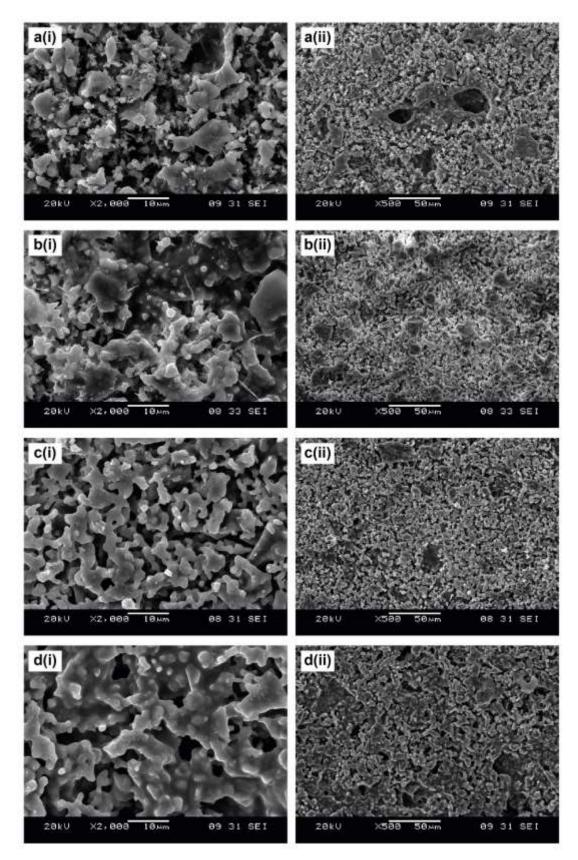
**Figure 6.** The morphology of sintered CaSiO<sub>3</sub> samples with X2000 magnification at (a)i) 1100°C, (b)i) 1150°C, (c)i) 1200°C (d)i) 1250°C, and with X500 magnification at (a)ii) 1100°C, (b)ii) 1150°C, (c)ii) 1200°C, (d)ii) 1250°C.
