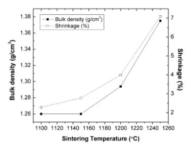
Figure 5. The effect of sintering temperatures on density and shrinkage.
