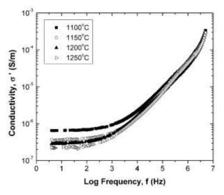
Figure 11. Frequency dependence of AC conductivity under 300°C for calcium monosilicate sintered at different temperatures.
