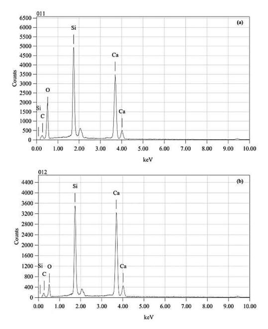
Figure 7. EDX spectrum from the (a) light and (b) dark area of the sample sintered at 1250°C.
