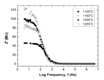
**Figure 10.** Variation of the real part (Z') of impedance with frequency under 300°C for calcium monosilicate ceramics sintered at different temperatures.
