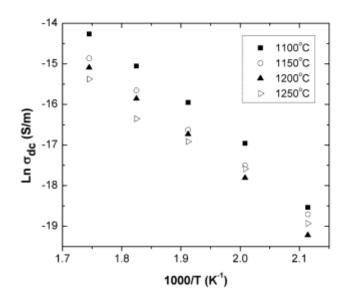
Figure 12. Arrhenius plots for the samples sintered at 1100°C – 1250°C.
