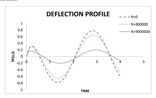
Figure 2: Displacement responses of a simply supported beam resting on an elastic foundation and subjected to an action of constant moving loads for various axial force, N and fixed value of foundation modulus K = 200,000.
