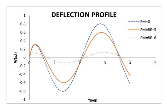
Figure 3: Displacement response of a simply supported beam resting on an elastic foundation and subjected to action of constant loads for various values of foundation modulus K and fixed value of axial force N = 200,000.
