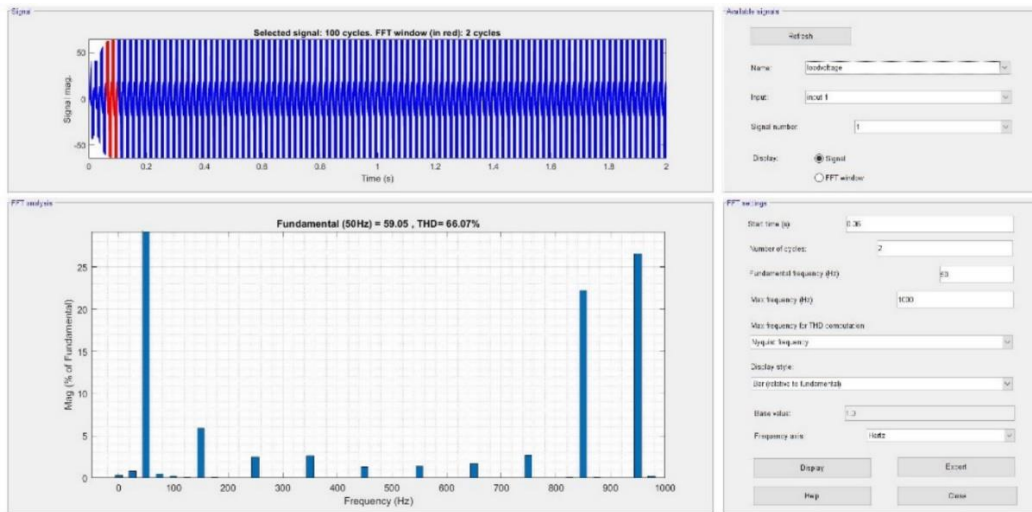
Figure 21. THD load voltage for single-level central inverter at partial shaded setup
