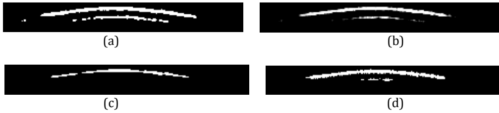
Figure 12. Output of filter processes towards Scan 1 data: (a) median filter, (b) average filter, (c) Gaussian filter, (d) Wiener filter
