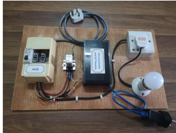
Figure 5. Prototype of the Remote Warning System for MCB Power Shortage via IoT.
