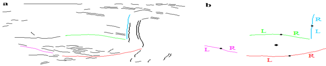
Figure 2.2(a): Edge fragments of a swan image, with four boundary fragments of swan, Figure 2.2(b): Four sample fragments extracted from image. Blue, green, red and magenta fragments have orientations [90, 90] , [0, -30] , [0, 30] and [-30, -60] . (Anvaripour and Ebrahimnezhad (2013))
