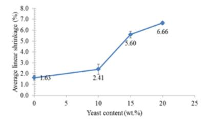
Figure 1 Average linear shrinkage against weight percentage of yeast content
