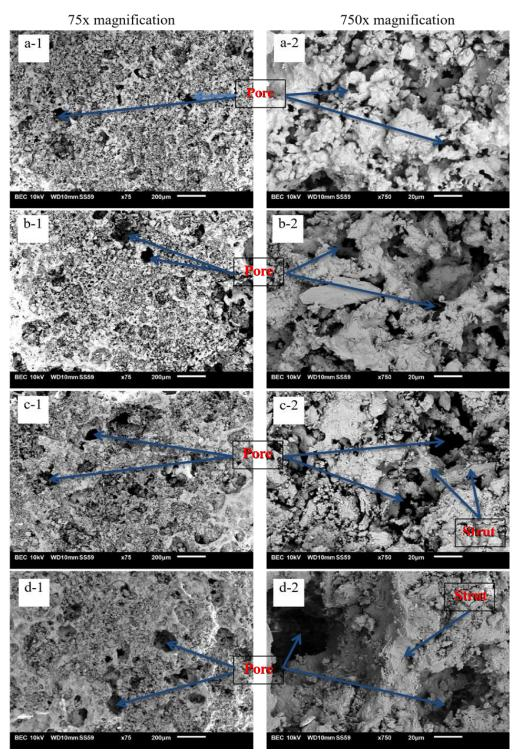
**Figure 3** Macrostructure of sintered porous ceramic: (a) 0 wt.%, (b) 10 wt.%, (c) 15 wt.% and (d) 20 wt.% at 75x and 750x magnification by using scanning electron microscope (SEM)
