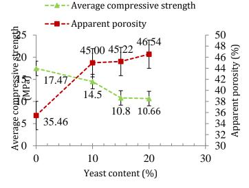
Figure 5 Relationship between average compressive strength and apparent porosity as functions of yeast content
