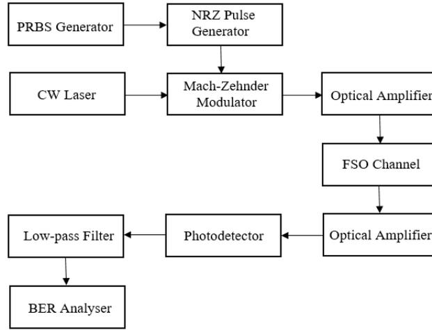
**Figure 2.** Block Diagram of FSO system
