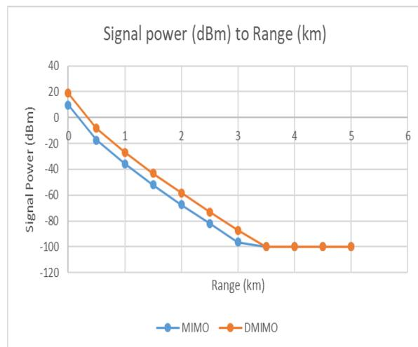
**Figure 12.** Signal power to range plot of MIMO and DMIMO system under moderate fog condition
