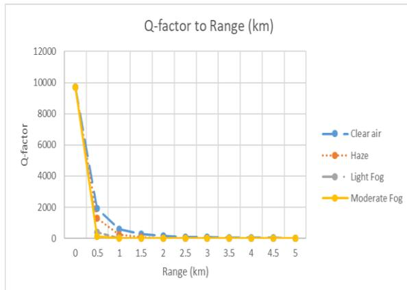
**Figure 9.** Q-factor to Range plot of MIMO FSO under different atmospheric conditions
