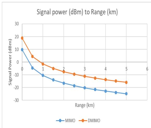
**Figure 11.** Signal power to range plot of DMIMO and MIMO system under clear air
