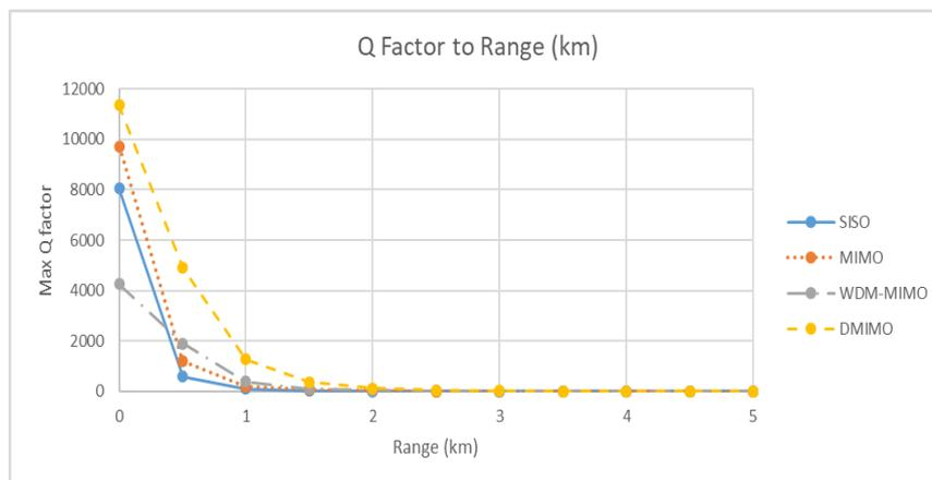
Figure 6. Q-factor to Range plot under atmospheric turbulence
