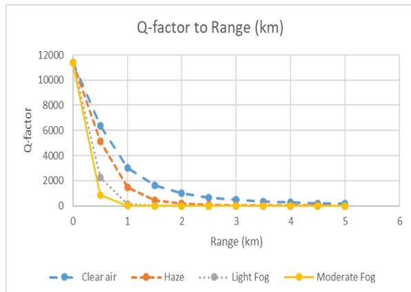
**Figure 10.** Q-factor to Range of DMIMO FSO system under different atmospheric conditions
