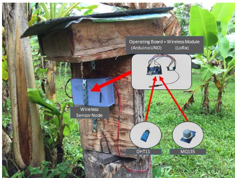
Figure 3. Placement of monitoring system at stingless beehive
