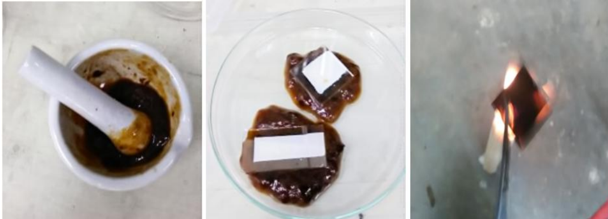
Figure 3. (a) Dye preparation (b) Coating process of the dye to the photoanodes and (c) Deposition of soot of candle carbon.
