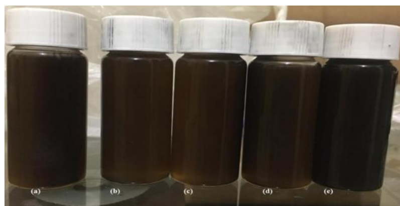
Figure 9. Photograph of (a) 0.1wt % (b) 0.2wt % (c) 0.3wt.% (d) 0.4wt.% (e) 0.5wt.% of nanofluid after one day.
